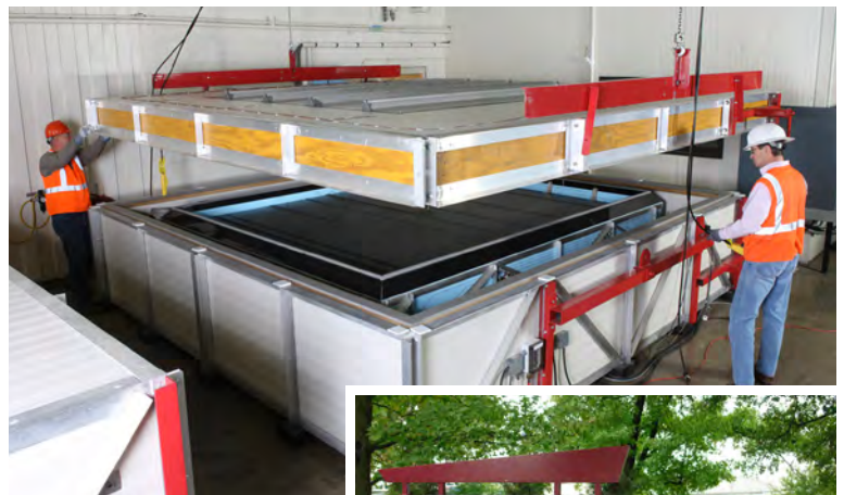
The IAS accredited Butler Guarded Hot Box is a state-of-the-art design that can accommodate 8'x 10' roof or wall sections fitted with up to 300 sensors to accurately measure temperature, humidity and air flow.
